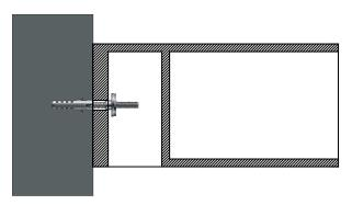
4. Place the basin in position against the wall, locating the fixing bolts through the holes in the rear of the basin. Push a plastic washer, followed by a metal washer, onto each fixing bolt.
