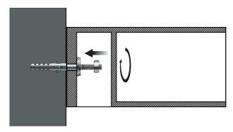
5. Screw a metal nut onto each fixing bolt to secure the basin. Caution: Do not overtighten, as this may damage the ceramic.
