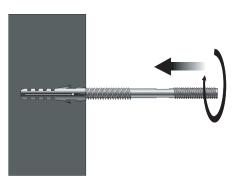
3. Screw a fixing bolt into each fixing plug using a 8 mm spanner until the spanner contacts the wall.
